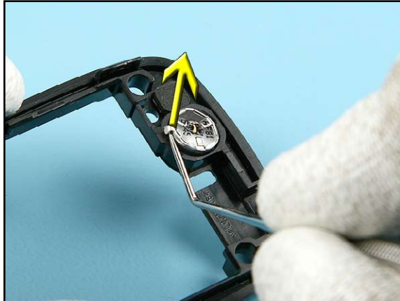
14. Remove the EARPIECE with the dental pick.
